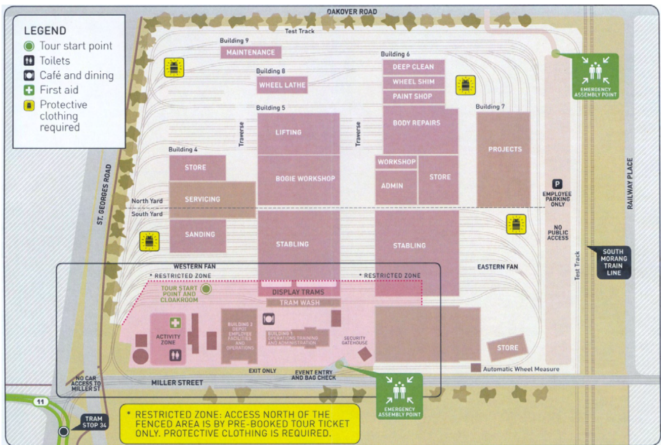
New Preston Depot and Workshops site plan provided by Yarra Trams on Open Day
