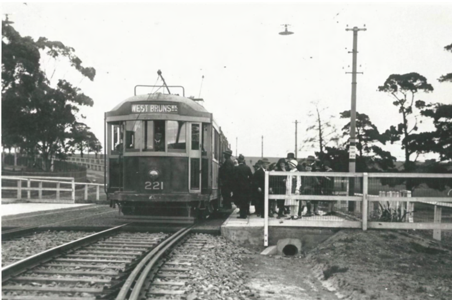
Tram 221, the third W class built, waits for passengers at the Zoo platform stop just south of the Melbourne to Fawkner railway embankment (c1925). Note the absence of a route number box on its roof and the picket fence around the Zoo.
