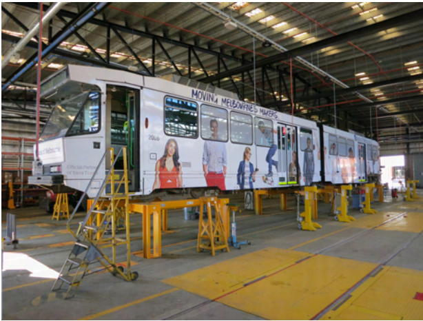
B2008 on mechanical hoists in the workshop
