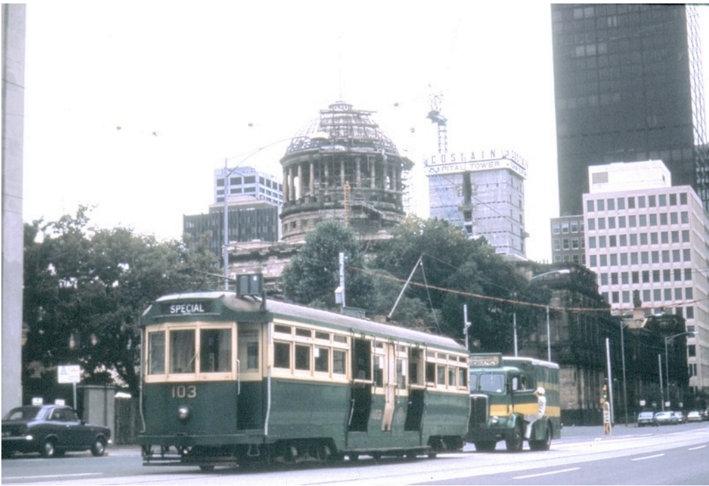
LEFT & BOTTOM LEFT: R10 recovery vehicle prepares to propel L103 along William St to Latrobe St because of weekend cut to power.
