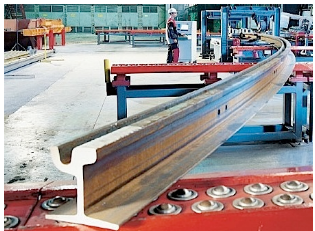
ABOVE: voestalpine Schienen GmbH applying the curve to grooved tramway rail. Photo: voestapline
