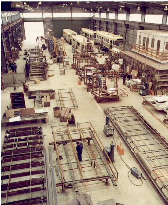
LEFT: Inside the Comeng factory, Dandenong showing the first stages of construction of A and B class vehicles and four nearly completed Z3 trams in the background (early 1980s). Photo: TDU collection
