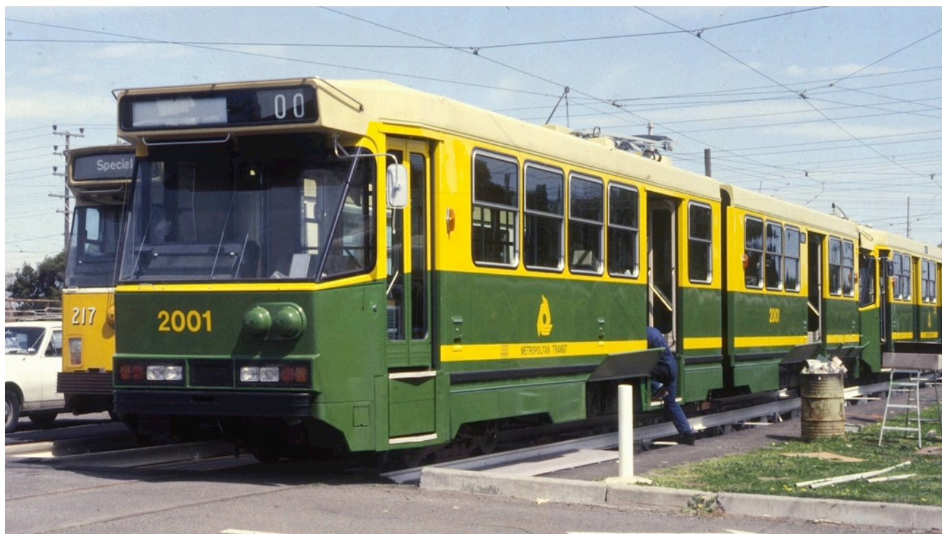
Melbourne's first light rail vehicle B1.2001 undergoing its many commissioning checks at Preston Workshops (8 October, 1984). Note the dual height doorway that was removed after trials. Photo: Trevor Triplow
