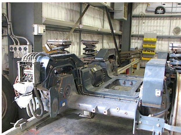
Siemens D class fixed truck at Southbank Depot showing the space for the central passenger aisle. (2011)
