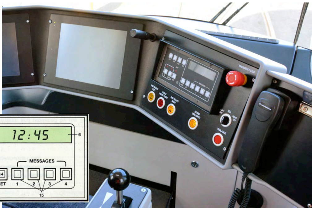
INSET: Diagram of the AVM control head from the driver's manual (c1989). Buttons 1, 2, 3 & 10 are for communications with the Operations Centre, PA (9) is for passenger announcements and TEST (11) self-tests all AVM functions before departing the depot. Several items of information were added to the default screen (6) in the 1990s.
