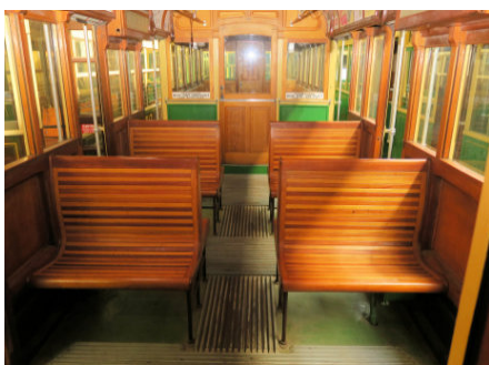
The three pictures above illustrate the evolution of the drop centre layout in the W class. W2 510 at left has the standardised layout of the W2 – note the narrow centre walkway. W5 774 has a much wider centre walkway enabled by the extra width of the car body. W7 1040 – the last W – opens up the drop centre by using longitudinal seats. All photographs by Mal Rowe at the Melbourne Tram Museum, January 2022.
