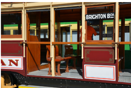
Victorian Railways drop centre tram number 41 has been restored to the appearance as built by Melbourne Tramcar Preservation Association. The stanchion gives an impression of a wide entrance, but the seat and seated passengers reduce the effective width. Photograph by Mal Rowe, 14 September 2014.
