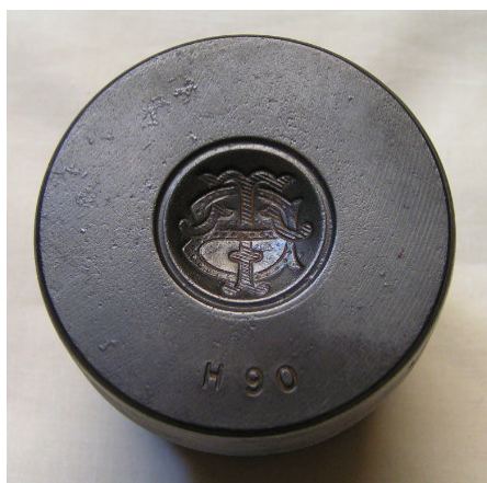
Female section of a two-part Stokes die for an M&MTB button. From the collection of Robyn Caddy.
