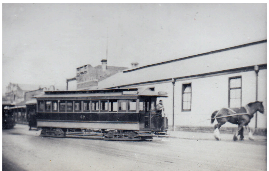
A 30-foot bogie car being hauled into the Brunswick car house/depot by horse (late 1920s). Photograph from the collection of the Melbourne Tram Museum.
